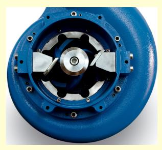
The high performance chopping mechanism ensures thorough maceration of slurry prior to entry into the impeller, reducing the risk of blockage. Shear pin protection of the chopping mechanism and independent sealing of both gearbox and pump casings ensures long and trouble-free working life.
