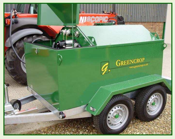
Greencrop offer a high speed bunded fuel (diesel) bowser for highway use. The high speed to version GCFB220T has a capacity of 1000 litres (220 gallon), with over 110% bund. It is fully compliant to ADR - IBC - UN approval, fitted with implosion and explosion safety valves. The unit also complies with the latest VOSA type approval regulations, IVA (individual vehicle approval) certification and current regulation lighting.
