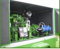
All models are manufactured at our assembly plant near Ely in Cambridgeshire using the highest quality materials and attention to detail, giving built-in reliability and a long-lasting finish. Greencrop pump sets use lveco industrial semi-electronic engines with a balanced crankshaft. These high torque engines give excellent fuel consumption and are well proven for use on irrigation pumps sets coupled to a Caprari MEC water pump.
