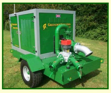
Two models, the GCEP125S and GCEP170S using Iveco N45 15HP and N67 170HP engines, encompass purpose designed engine and pump management systems to allow for either automatic pressure maintenance, enabling the operator to specify a required pump outlet pressure where the controller will modulate the engine speed to maintain the required pressure, or remote throttle control via radio telemetry. All Greencrop controllers include full engine protection and auto start facilities.
