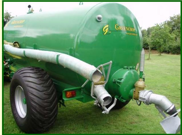
Greencrop Tankers are quality British Manufactured. The tanker barrels are rolled from high quality 6mm and 8mm steel plate.
